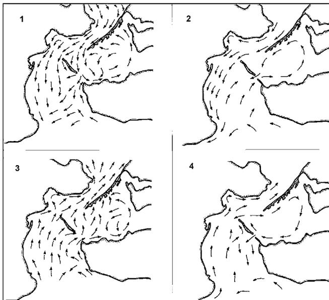
**Fig. 3.6a.** The Kerch Strait water flows impacted by the Northern wind flow (Azov) are given above, and the Southern wind flow (Black Sea) is given below; before construction of the Tuzla dyke (left) and after the construction (right) as observed in autumn 2003.
